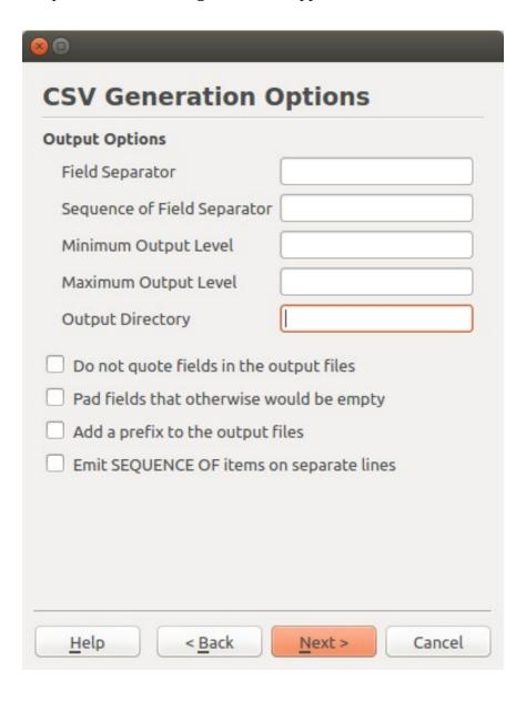
Unlike XML output, CSV output is always directed to a file (or, more likely, several files). The output in the compilation window is therefore a little different than what is seen when XML output is selected without an output filename. This behavior is normal.
