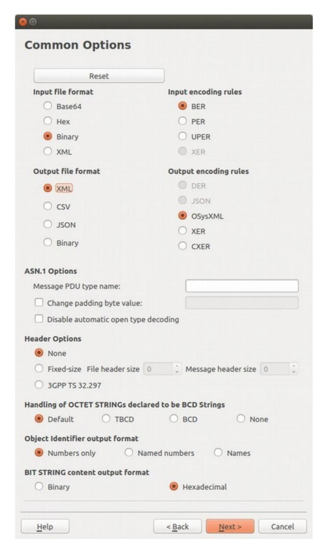
Within the input and output groups of radio buttons, selecting certain options will cause some options in the other box to be disabled. The Reset button at the top will re-enable all radio buttons and will show none of them selected.
