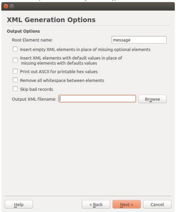
Users have two options for how to direct their XML output: it can be dumped to the GUI directly or else to a file. When the XML output filename is not provided, users will see the decoded XML output in the compilation window.
