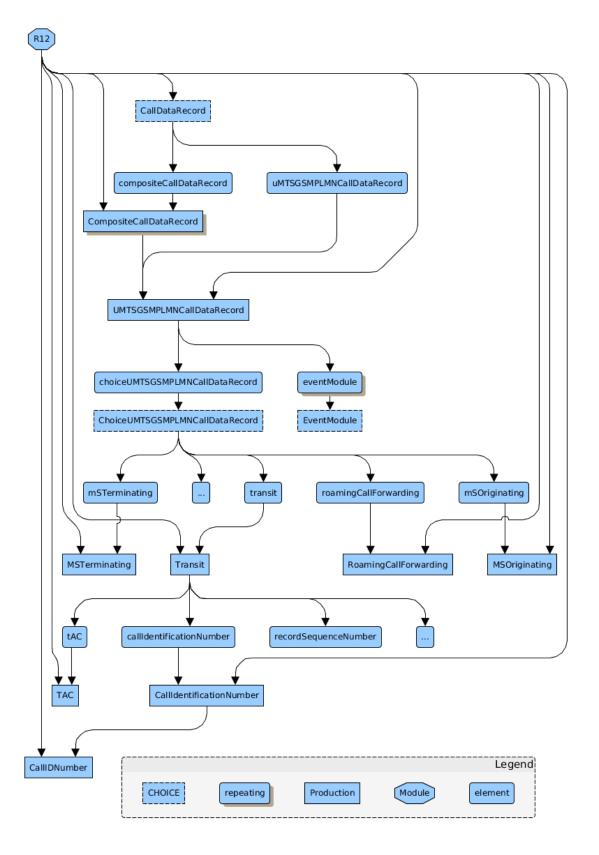
Using -minLevel 3 on the command line produces one output file for each CDR: R12\_UMTSGSMPLMNCallDataRecord\_MSTerminating.csv and others, as seen in this example execution:
