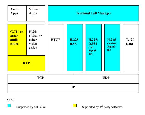
In this diagram, parts of the H.323 stack supported by OOH323C are shown in the light blue color. In addition, sample programs are included that contain third-party open-source media code to demonstrate a complete audio application that can play and receive a recorded audio file. The additional parts of the stack supported by this code are shown in yellow.
